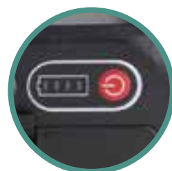
super touch switch LED battery indicator
